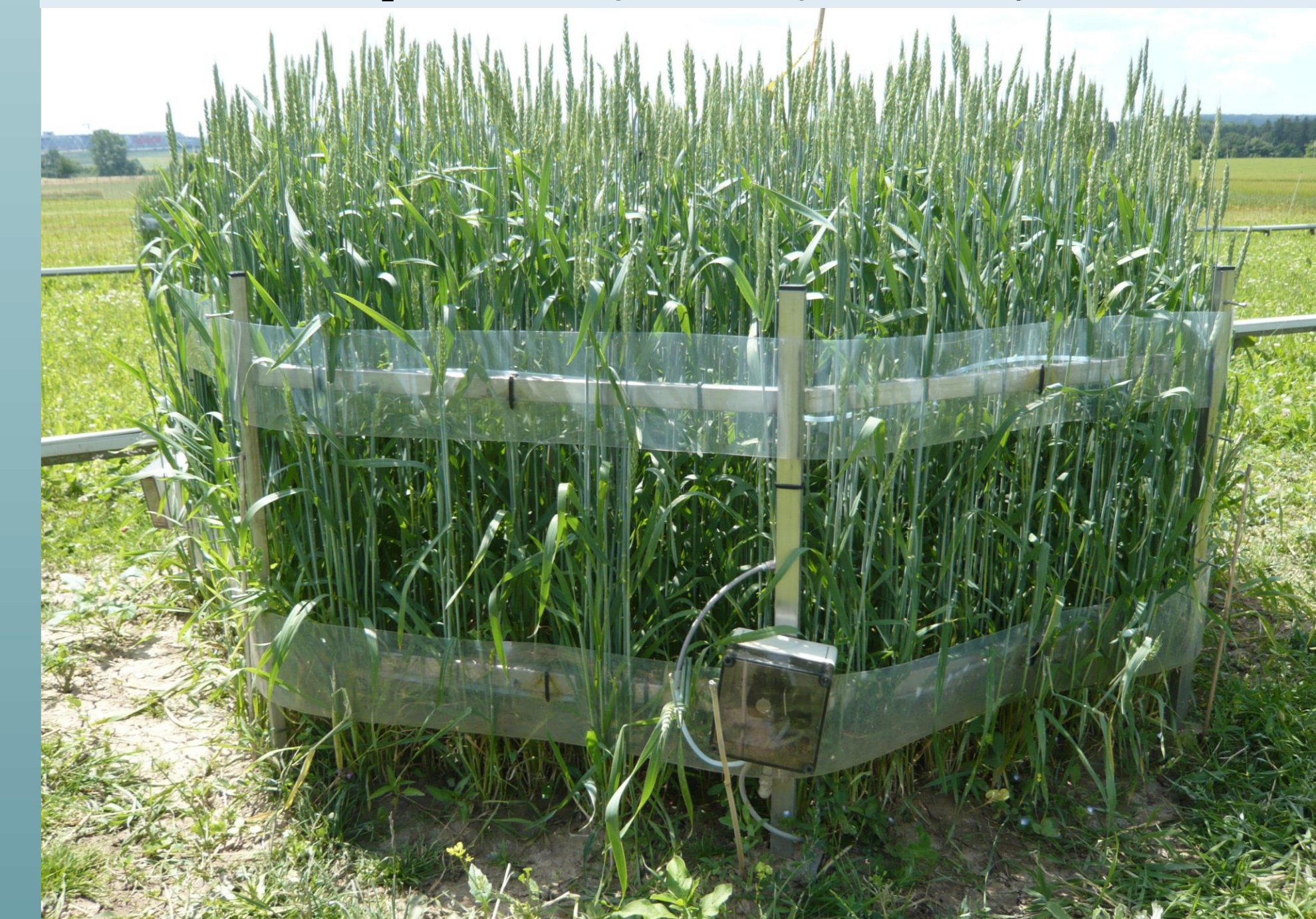
Mini-Free-Air CO 2 Enrichment (mini-FACE) at University of Hohenheim
